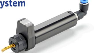
The new innovative *CIM* clamping system provides high precision and repeatability of the Tiny Tools cutting edge, as well as fast and easy tool exchange without removing the holder. The *CIM* system includes an internal tool indexing mechanism which index the tool in the correct orientation, as well as strong and rigid collet clamping for high stability.
